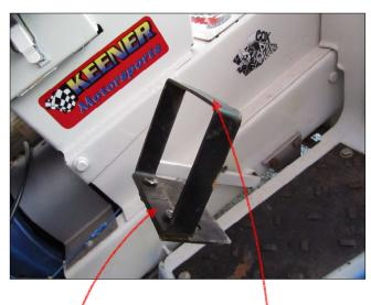
With a Pedal Extender in place, a puller can now opt to place their foot directly on the pedal (original position)...or...place their foot on top of the pedal extender.
